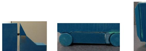
Figure 1: (From Left to Right)- Tractor Top, Trailer Side Skirt, and Boat-tail Trailer Door.
