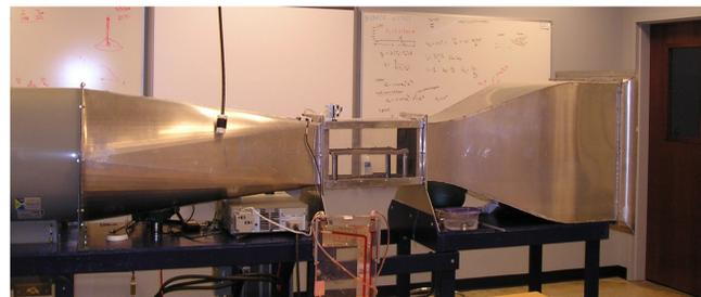
Figure 4. Wind tunnel that was used to produce air flow
