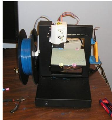
Figure 2: 3-D Rapid Prototyping Machine used to print tractor-trailer
