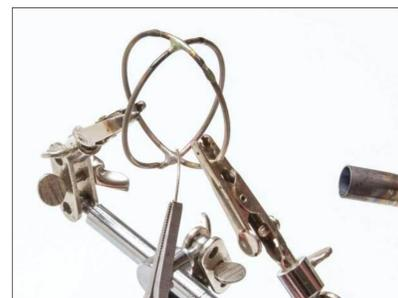
Left: Specialists at Make Magazine soldering (technically brazing) together the inner grid using MAAP gas and silver filler metal.
