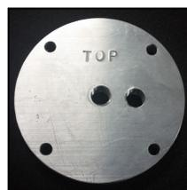
Left: Top flange with ports machined for vacuum supply and vacuum gauge.
