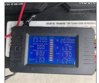
Figure 2: DC Multifunction Battery Monitor Meter
