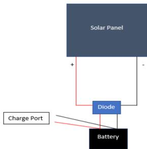
Figure 1: Final Design Wiring
