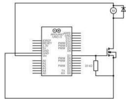
Figure 2. Air Pump Control Schematics
