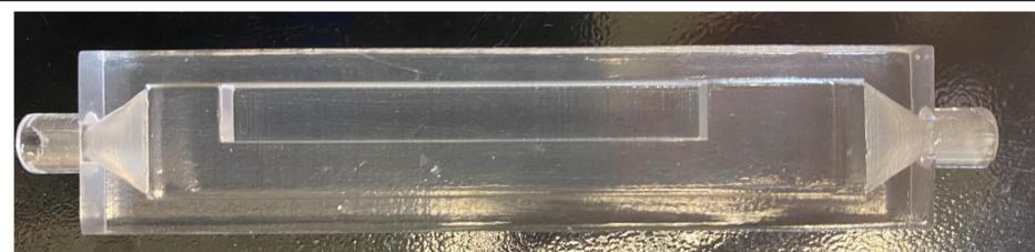
Figure 2. The 3D Printed SLA Flow Chamber with a Hydrogel Reservoir
